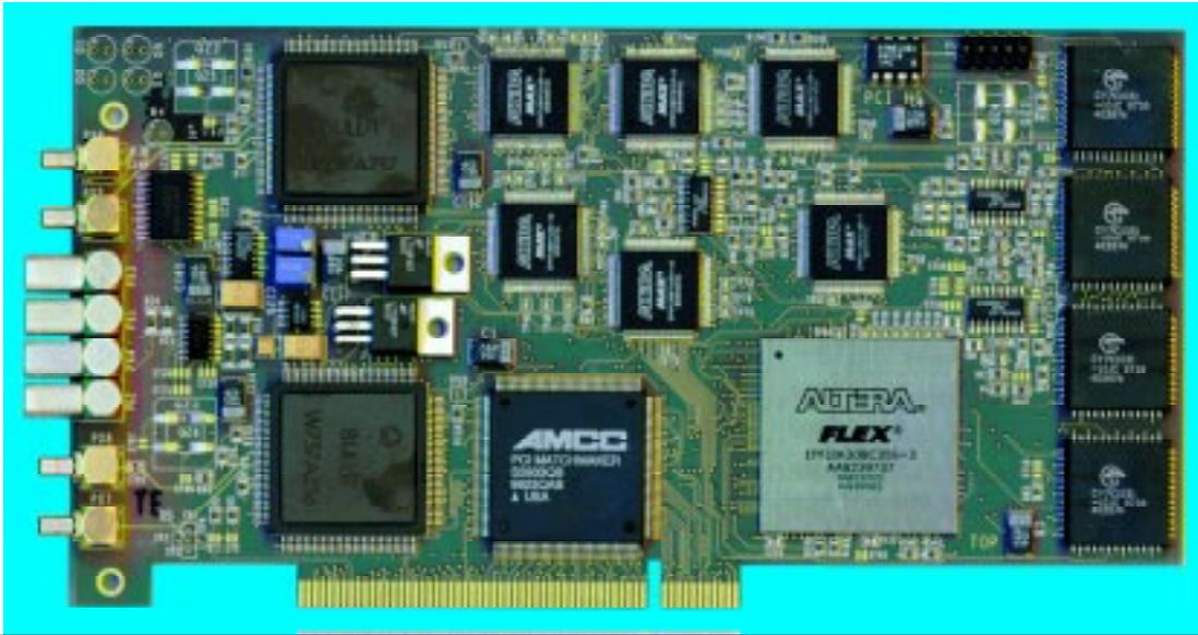
Fig. 12. Photograph of the PCI HS-link Interface
