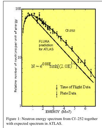
The test was performed at the National Institute of Standards and Technology (NIST) in Gaithersburg Maryland using a Californium–252 fission source which produced  $5.0 \times 10^9$  n/s. The test exposure lasted for 3 weeks; a period short compared to the 2.65 year half-life of Cf–252.
