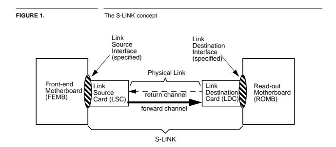
In many applications a uni-directional data channel will be required. In other cases the user might require to send flow control and other information back to the FEMB. The S-LINK, therefore, can be constructed in either a *simplex* or a *duplex* version.
