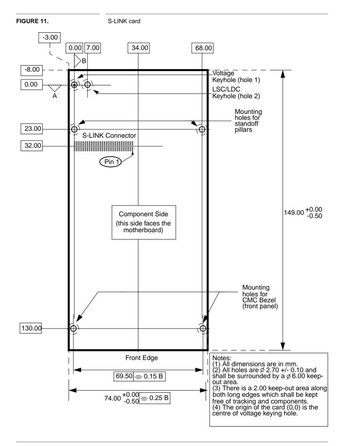
**3.** The connector is a 64-pin surface-mount CMC connector and is a plug on both S-LINK cards (LSC and LDC) and a receptacle on both motherboards (FEMB and ROMB). Drawings of the surface mount pad layouts for the connectors are given in Figure 12 and Figure 13.
