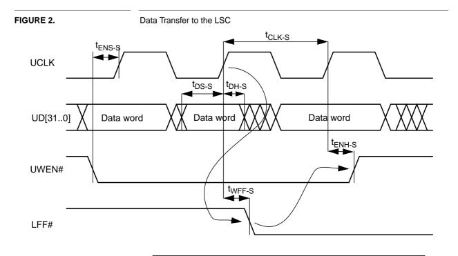
Note: In this diagram, only one extra data word is transferred after LFF# goes low. In fact, up to two words may be transferred.
