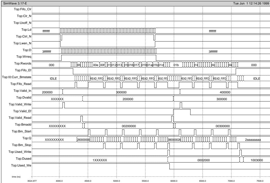
**Figure 7: Handling of an event spanning over two memory pages (page sizes and event size values used are just demonstrating the capability of the state machine and are not the final ones).**
