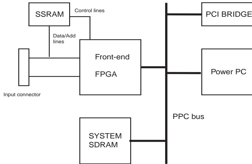
**Figure 1: MFCC block diagram (current release, only the blocks relevant to FE, the connection of the FE-FPGA to P2 is not shown).**
