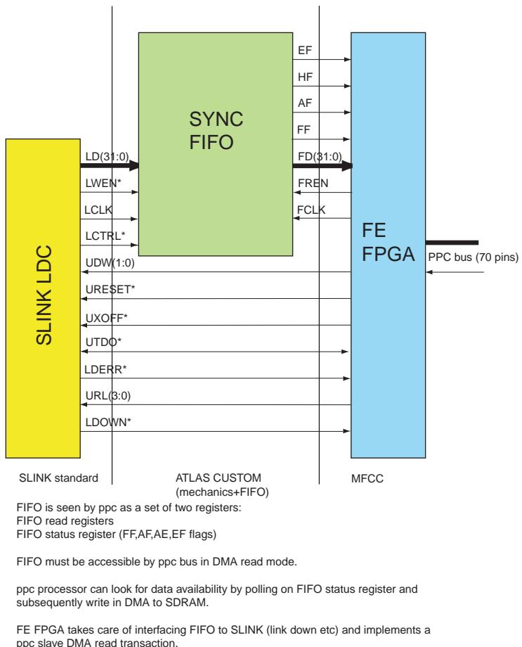
**Figure 2: July solution for interfacing LDC to MFCC.**
