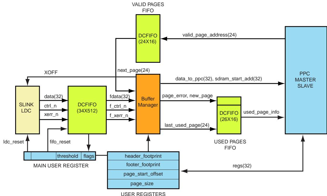
**Figure 4: Master-ppc FE-FPGA block diagram**
