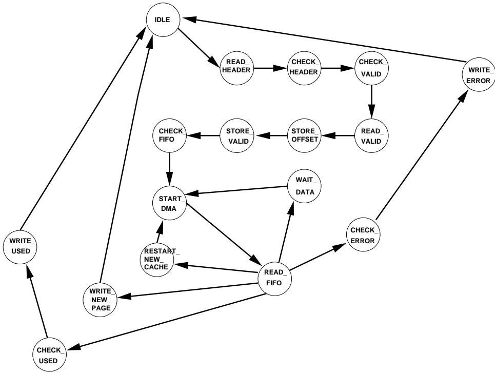
**Figure 6: buffer\_manager state machine block diagram.**
